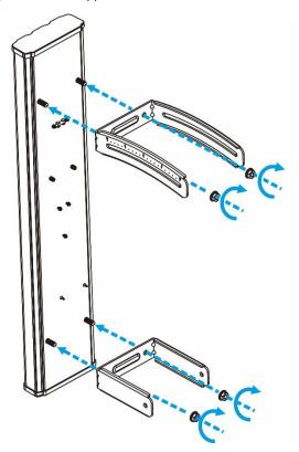
(2) Secure the two fastening pieces to the upper and lower brackets with four screws, two for each.
