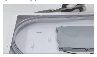
(5) Split the optic fiber from the copper cable of a hybrid cable. Peel off the outermost sheath of the copper cable by 30 mm (1.81 in.) to 50 mm (1.97 in.). Peel off the sheaths of the two wires in the copper cable by 5 mm (0.20 in.) and crimp them into the wire holders in sequence. Then gently pull out the wires to ensure that they are securely connected.
